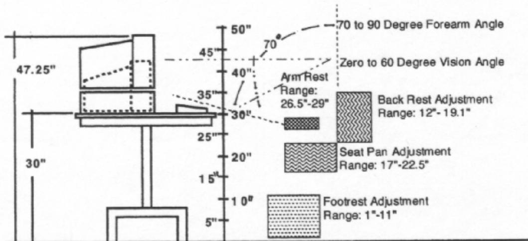
Figure 1. A 2-D Analog Recommending Adjustment Ranges for Proposed Seating Using the Forearm Model
