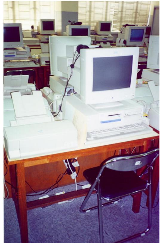
**Figure 1: Typical computer set-up in a local secondary school computer laboratory. The 3-tier system consists of the display screen on top of the CPU which is on top of a metal frame housing the slideout keyboard tray. The table has just enough room to hold the computer and the printer. It is not clear where the student would place the mouse. The chair used is a non-adjustable fold-up chair.**
