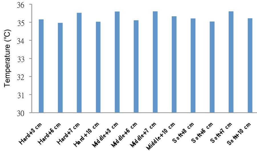
Figure 3. The average temperature measures of the 12 mattress toppers.
